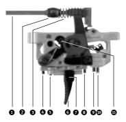
The sear engagement is too long: There is a small distance between the second stage and the release of the trigger.
